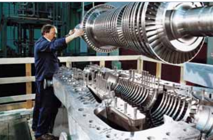
10 12 MW backpressure turbine
