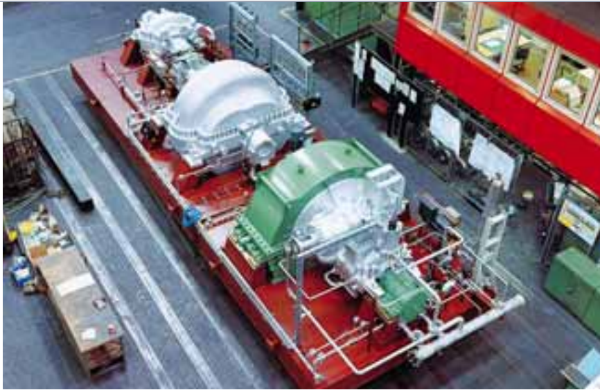
31 Compressor train with condensing steam turbine
