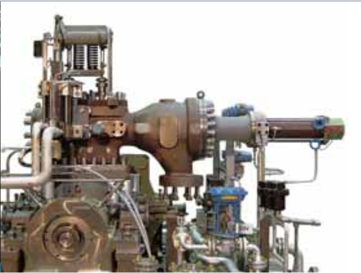
21 Steam turbine upper section with flanged steam chest
