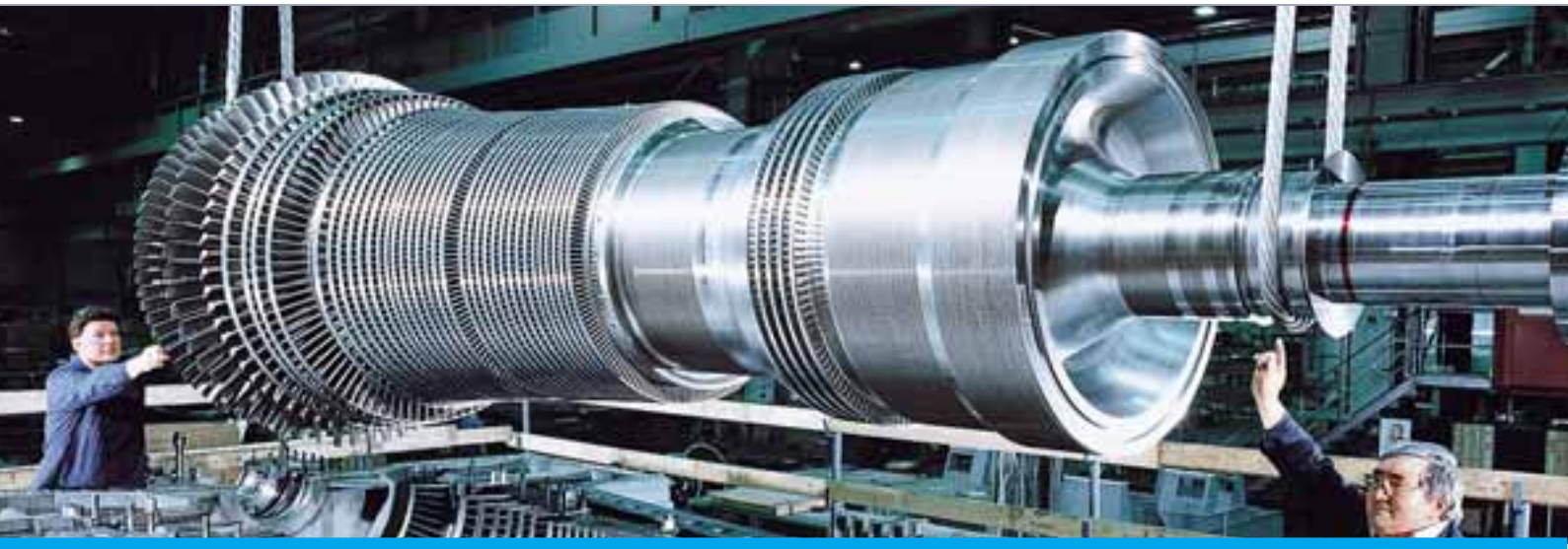
15 Central admission turbine during assembly
