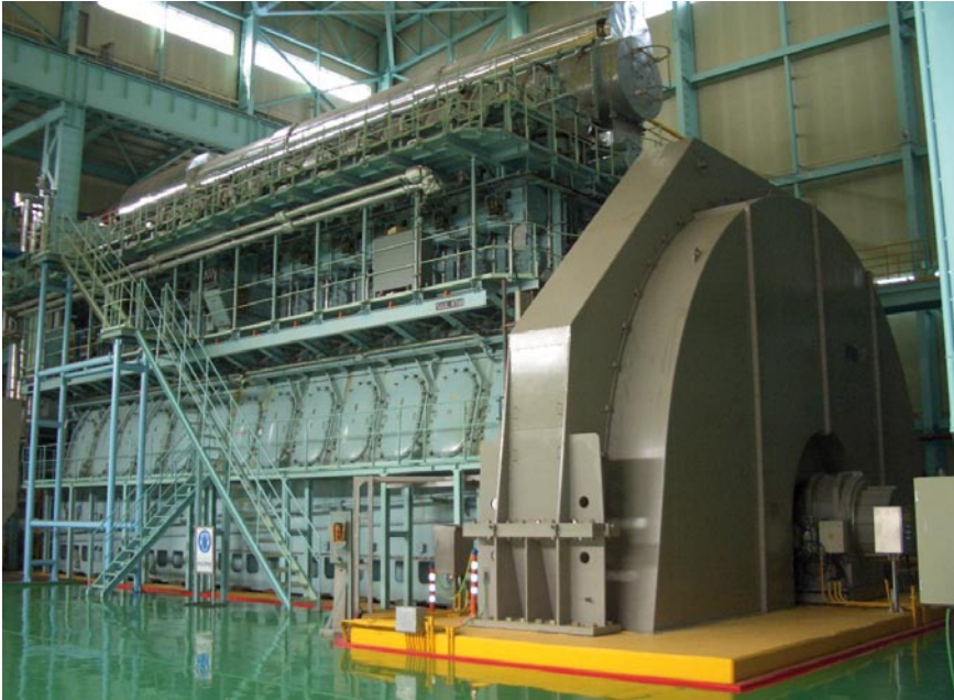
Fig. 16: MAN B&W 12K80MC-S at Buk Cheju, Korea Midland Power
